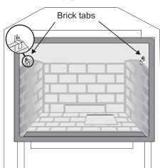
Note: If the bottom brick panel must be removed: Remove the Rear Log Stand, then remove the Burner Tray. See the instructions in the "Removing Valve" section.
